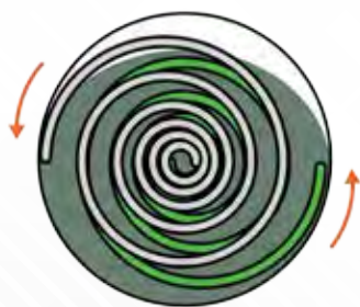
Scroll Compression Diagram
